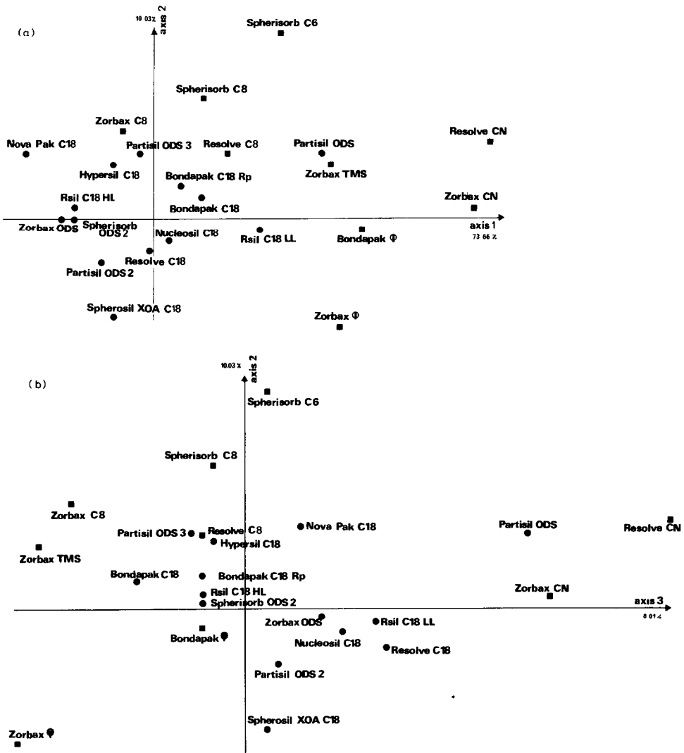
Fig. 2. Results of correspondence factor analysis of capacity factors of 63 solutes in 23 RP-HPLC systems. Projection of 23 RP-HPLC systems on to the plane defined by (a) 1 and 2 main axes of inertia; (b) 2 and 3 main axes of inertia. ●, Systems with ODS packings; ■, systems with C 8 , C 6 , TMS, CN and phenyl packings.
